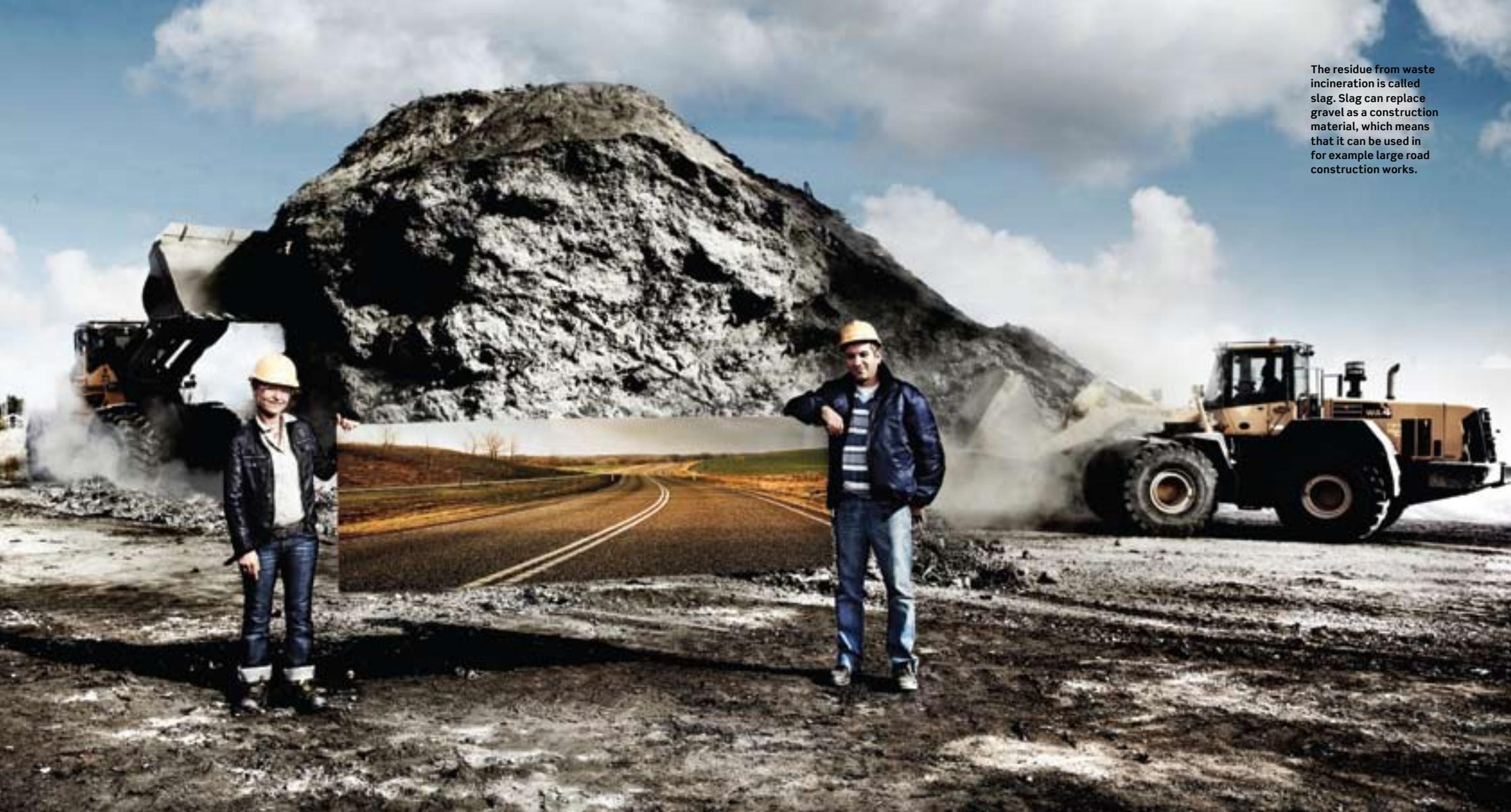
The residue from waste incineration is called slag. Slag can replace gravel as a construction material, which means that it can be used in for example large road construction works.
